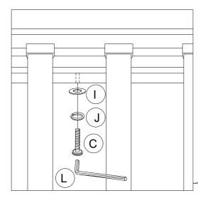
Check that the frame is central by adjusting the alignment of the frame and brackets before fully tightening all bolts. The metal frame should not contact the faux leather at any point.
